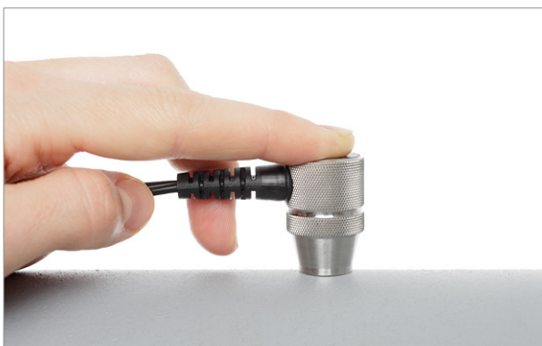
Wall thickness gauge NT in use
